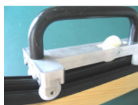
notching of the continuous gasket
