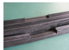
notching of the abutting gasket
