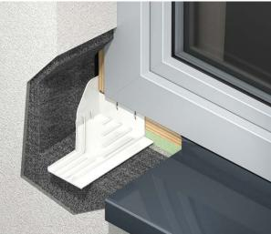
No advance planning is required to install the component, which matches the GUTMANN GS 40/GS 25 window sill system. It is simply attached to the facing frame on the outside of the window. Installed below the window, it reliably channels any moisture that penetrates the construction to the outside, thus preventing costly structural damage.
